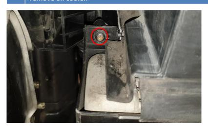
2. Loosen the Torx T40 screw that holds the oil lines to the oil cooler. Have an oil pan underneath and remove lines from oil cooler. Use the included silicone caps to plug the oil lines during oil cooler swap to minimize oil leak.
