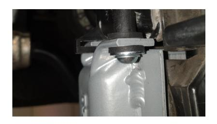
5. Install the supplied o-rings on the oil pipes and connect them to the oil cooler and tighten the Torx T30 screw.
