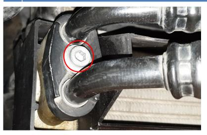
4. Install do88 oil cooler using supplied accessories, on each side 1 x 6x25 Screw, 1 x flat washer, 2 x rubber washers and install according to picture.
