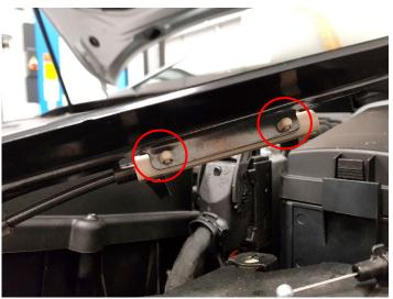
**12.** Remove 3x Torx T30 screws for both the head lights. Then remove both headlights by gently pulling them forward and disconnect the cable connector.
