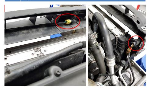
**15.** Disconnect the cable connector for radar, temperature sensor and both horns. Make sure to loosen all wires from the radiator support so it can be removed from the car.
