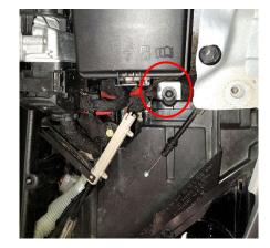
**13.**Remove the air intake scoop by removing 2x Torx<br/>T25 and disconnect the radiator hose from clips.
