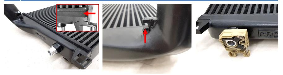
25. If your radiator does not fit in the lower slots of the do88 intercooler, you may need to trim the plastic tab on the OE-radiator marked on the photo below. Use a cutting pliers to remove most of the plastic tab. Then carefully grind the remaining residue until surface is flush.
