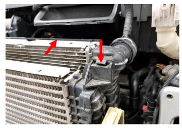
24. Tape the included 5mm thick sealing strip on the outside of the welding line on both sides according to the photo below. On both lower radiator brackets put a piece of the included 4mm thick self-adhesive rubber strip according to photo below. Remove the OEM intercooler brackets and install them on the do88 intercooler.
