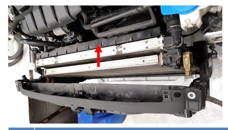
23. Release the radiator from the intercooler. Press the plastic tabs downwards on both sides while gently pushing the radiator backwards. Lift the intercooler out of the car.
