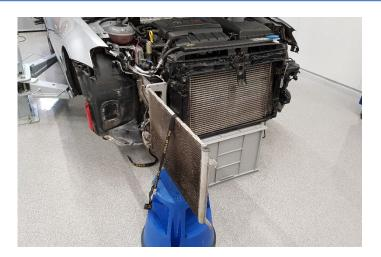
Lean the intercooler assembly towards the engine. With the help of a friend lift the assembly upwards from the radiator support frame. Then remove the radiator support frame.
