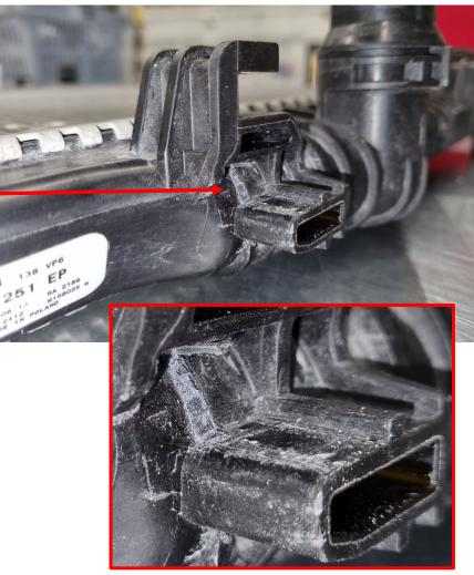
**26.** Cut the top right bracket on the AC-condenser. Cut on the outside of the raised rib.
