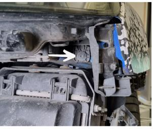
Remove 1x Torx T30 that holds the headlight. Do this on both sides of the car.
