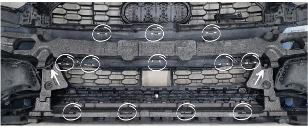
Install the ACC and outside temperature sensor. Use the 2x included stripes to secure the cables along the crash bar.
