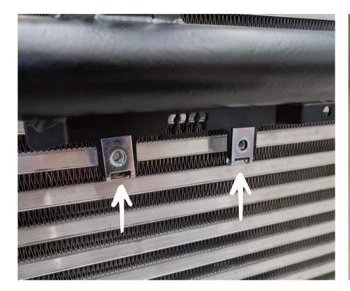
Install the 2x included M6 reed nuts as shown on picture.
