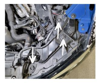
Step 10 Remove 3x Torx T30 that holds the headlights. Do this on both sides of the car.
