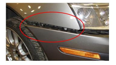
Remove the headlights by removing 3pcs of 10mm (on facelift 2pcs 10mm & 1pc 8mm) hex screws on each headlight and then pull/lift forward so you can disconnect the electrical connector from the headlight and then remove headlight from vehicle.
