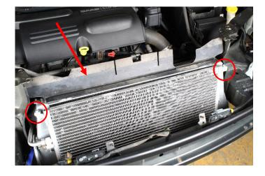
Remove the air guides on both sides of the intercooler by gentle pry out the tabs in the washer and then remove from intercooler pin.
