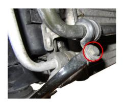
14. Loosen the 10mm hex nut just a bit, the remove the 10mm hex head screw from the bracket and then turn the bracket out from the car.
