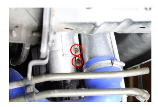
17. Loosen both hoses from intercooler by loosen hose clamps (with a 7mm hose clamp screwdriver or 7mm hex socket) and pull them off the intercooler connections.
