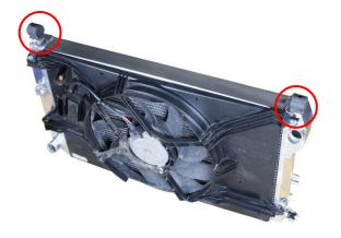
With the help of a friend lift the radiator while you remove the two bottom radiator brackets 2x E14 Torx.
