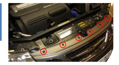
**4.** Remove the 4pcs of 8mm hex head screws marked on picture.
