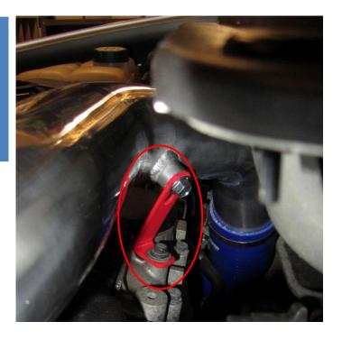
7. Install the hose/hoses on the inlet pipe hose nipples by pushing them in place.
