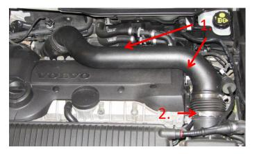
2. Loosen the hose clamp from turbocharger inlet. It might be hard to reach depending on which direction the clamp screw points. In some cases it might be easier to reach from underneath the car.
